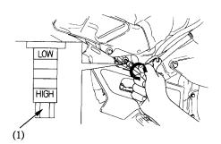
To reduce preload-turn the adjuster counterclockwise.
