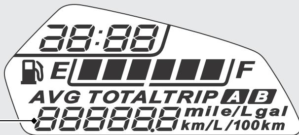
**Odometer [TOTAL] & Tripmeter [TRIP A/B] & Fuel mileage meter & Fuel consumption meter**
