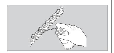
Do not use a steam cleaner, a high pressure cleaner, a wire brush, volatile solvent such as petrol and benzene, abrasive cleaner, chain cleaner or lubricant NOT designed specifically for O-ring chains as these can damage the rubber O-ring seals.
