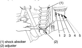
The spring pre-load adjuster (2) has 5 positions for different load or riding conditions.
