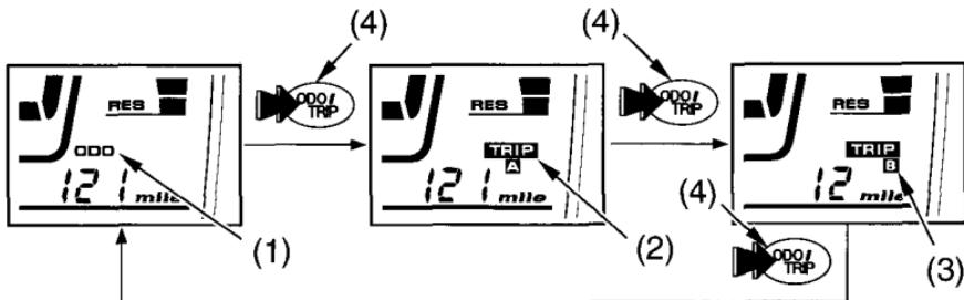
To reset the tripmeter to zero, press and hold the RESET button (5) for more than 2 seconds with the display in the tripmeter A or tripmeter B mode.
