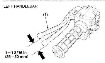
(1) rear brake lever/parking brake lever
