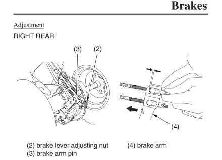
Adjust the freeplay of the rear brake lever/parking brake lever with the front wheels pointed straight ahead.
