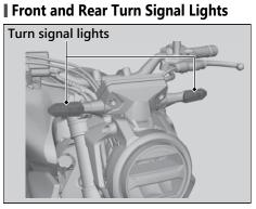
The front and rear turn signal lights use several LEDs.
