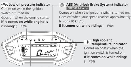
PGM-FI (Programmed Fuel Injection) malfunction indicator lamp (MIL)
