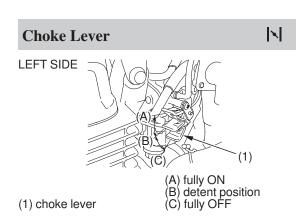
The choke lever (1) is used for starting the engine (page 29). The choke increases the percentage of fuel in the fuel/air mixture delivered to the engine.
