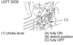
1. Pull the choke lever (1) up all the way to fully ON (A).
