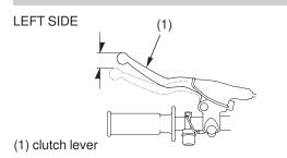
Inspection Check freeplay. Freeplay: 3/8-13/16 in (10-20 mm)
