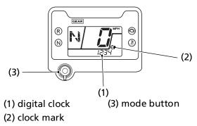
After the battery is reconnected (page 185), check the clock. Readjust the clock if necessary.
