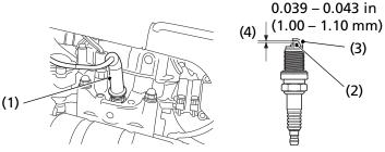
(1) spark plug cap(2) center electrode
