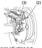
(2) brake lever adjusting nut(3) brake arm pin
