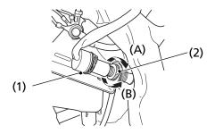
(1) rear brake light switch (2) adjusting nut
