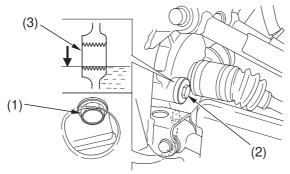
(1) oil drain bolt(2) oil fill cap
