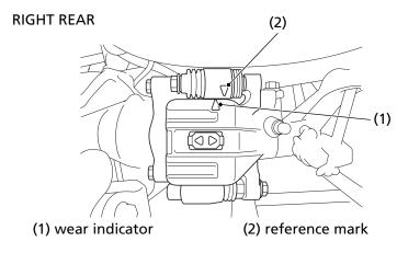
Check the wear indicator (1). If the wear indicator aligns with the reference mark (2), both pads must be replaced, see your dealer for this replacement.
