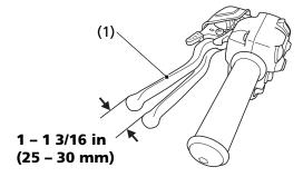
(1) rear brake lever/parking brake lever
