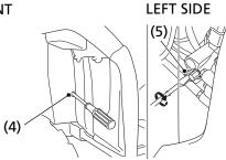
(4) emergency valve access hole (5) emergency valve
