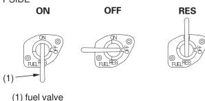
The manual fuel valve (1) is located on the left side under the fuel tank.
