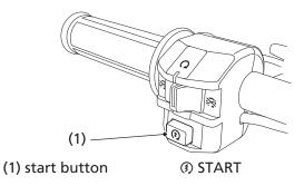
The start button (1) is used for starting the engine. Pushing the button in starts the engine. See Starting Procedure, page 56.
