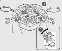
**5** Press the start button with the throttle completely closed. Release the start button as soon as the engine starts.
