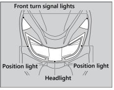
The headlight/front turn signal lights/position lights use several LEDs.
