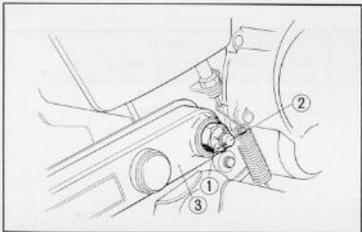
Fig. K4.4 ① Self-locking nut    ③ Rear fork
