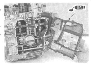
Carefully install the oil pan and tighten the flange bolts in a crisscross pattern in 2-3 steps.
