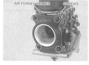
Remove the air funnel from the holder. Remove the O-ring from the carburetor body.
