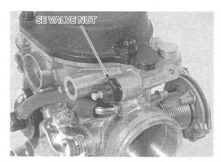
Remove the SE valve and spring.
