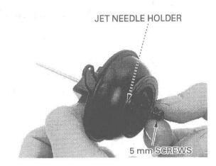
Remove the spring and jet needle from the vacuum piston.
