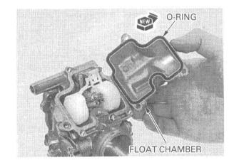
Install and tighten the three float chamber screws.
