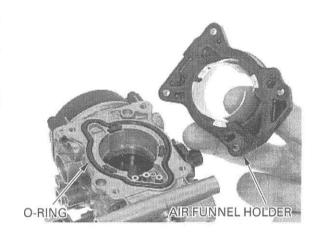
Install and tighten the holder screws.
