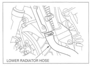
Remove the radiator mounting bolts. Remove the radiator from the right side.
