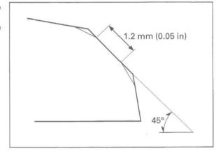
The location of the valve seat in relation to the valve face is very important for
