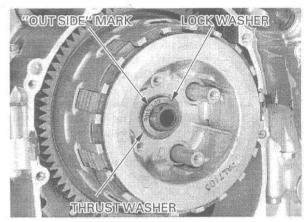
Apply oil to the new clutch center lock nut threads, then install it onto the mainshaft.
