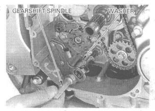
Remove the shift drum center bolt, shift drum center and dowel pin.
