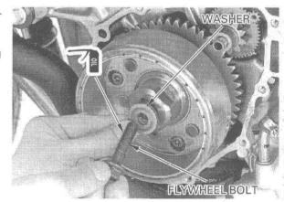
Hold the flywheel using the flywheel holder, then tighten the bolt to the specified torque.
