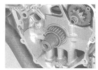
Install the flywheel aligning the key way in the flywheel with the woodruff key on the crankshaft.
