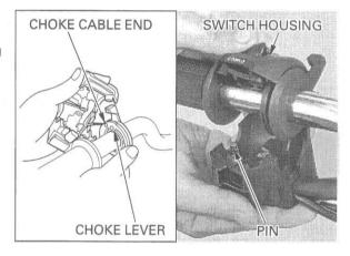
Tighten the forward screw first, then the rear screw.
