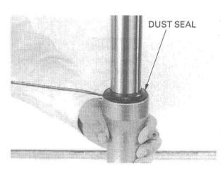
Remove the oil seal stopper ring.
