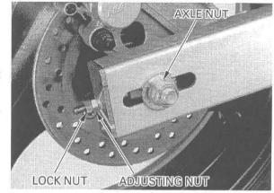
Remove the axle nut, washer and rear axle washer.
