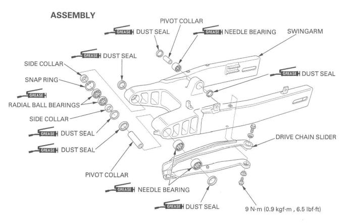
Apply grease to the dust seal lips, then install the dust seals and pivot collar into the shock absorber pivot.
