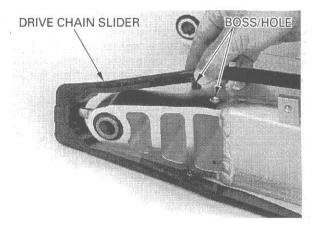
Install the collars and bolts, then tighten the bolts to the specified torque.
