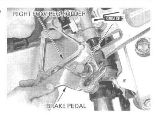
Install the washer, then install the snap ring into the groove securely.
