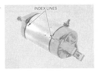
Install and tighten the motor case bolts securely. Apply clean engine oil to the new O-ring. Install a new O-ring onto the starter motor boss.
