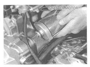
Install the ground cable and tighten the starter motor mounting bolts.
