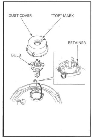
Install the headlight unit and tighten the screws securely.
