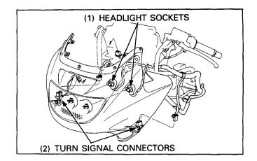
Remove the screws and turn signal unit. Remove the bolts and headlight unit.
