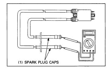
If the measured value out of the specification, remove the spark plug caps from the spark plug wires and measure the resistance between the spark plug wires.
