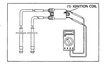
Measure the resistance between the spark plug caps.
