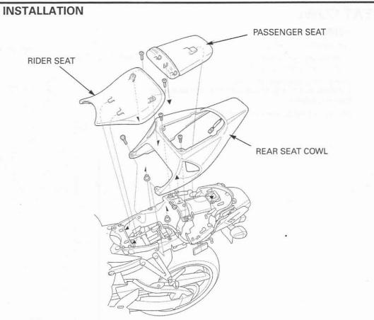
Make sure that the Conn mating surfaces of Instal the cowl bottom fender are seated onto the ness. rear fender properly before tightening the bolts.
