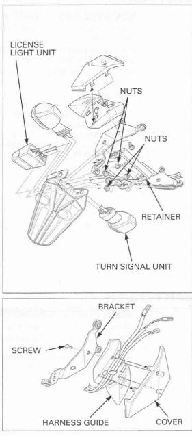
Remove the screw and left rear fender bracket, harness guide and cover.
