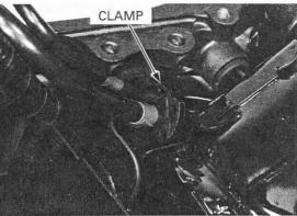
Remove the rear fender B-to-heat protector trim clips.
