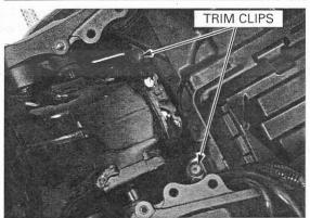
Remove the rear fender B from the seat rail.
