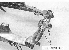
Replace the seat Assemble the seat rail by installing the seat rail rail as an assembly. assembly flange bolts/nuts.
