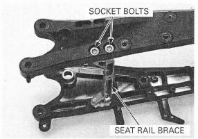
Remove the seat rail assembly bolts/nuts, then separate the right and left seat rail.
