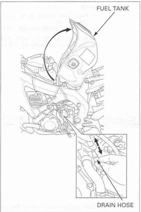
Support the fuel tank using a suitable support as shown.
